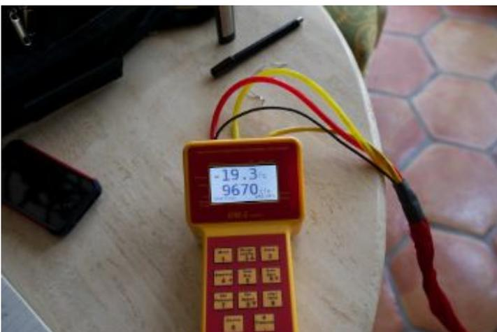
We could not get to -50Pa due to excessive leakage of air.
